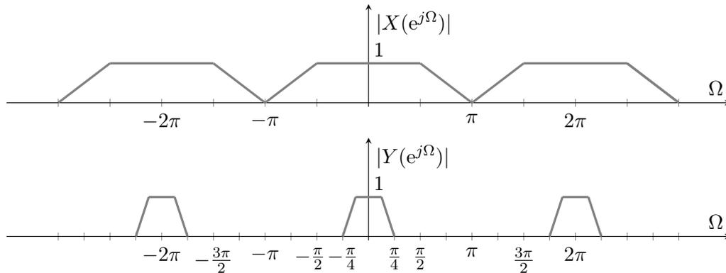
Figure 1: Input and output spectra of a multi-rate system.
