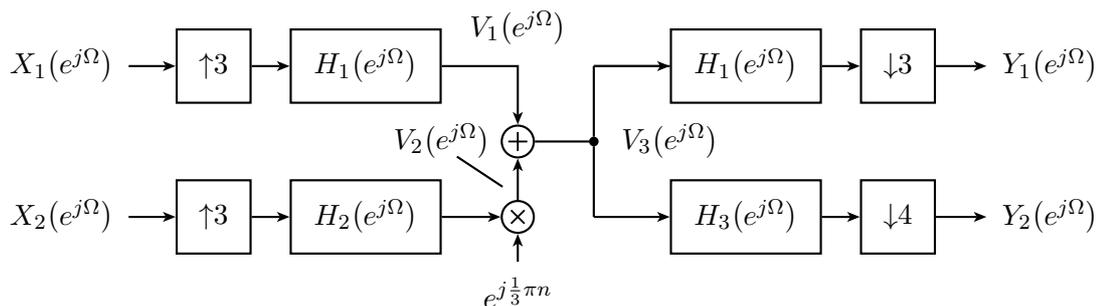
Figure 2: Block diagram of a multi-rate system.
