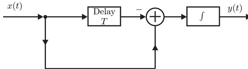
Figure 1: Hold circuit realization with a summer and an integrator.
