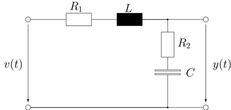
Values:  $R_1 = 100 \text{ k}\Omega$ ,  $R_2 = 100 \Omega$ ,  $C = 10 \text{ mF}$ ,  $L = 3 \text{ mH}$
