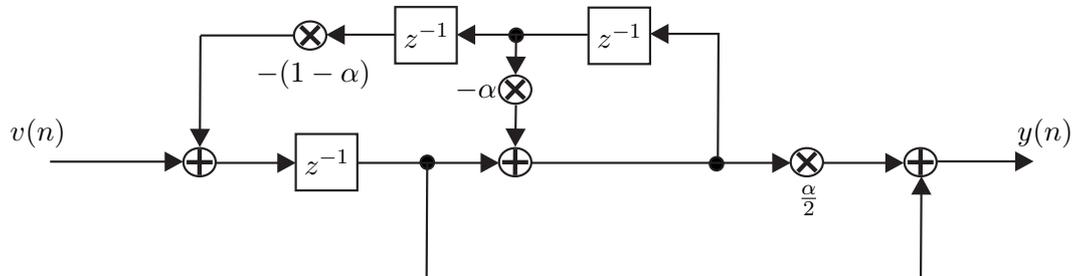
Figure 1: Signal flow graph of the system  $H(z)$ .
