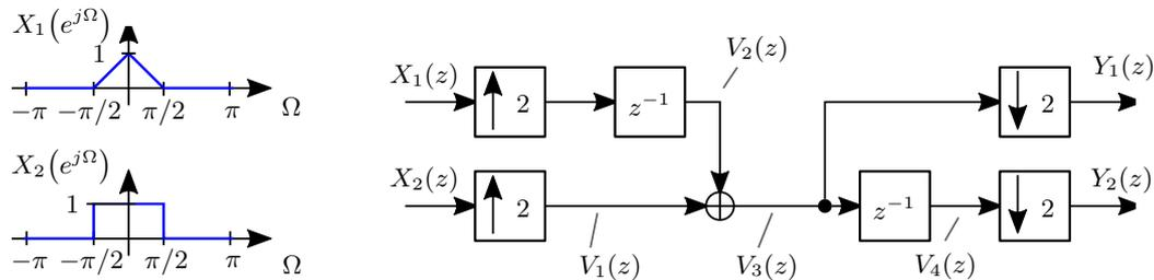
Figure 3: Block diagram of a multi-rate system.
