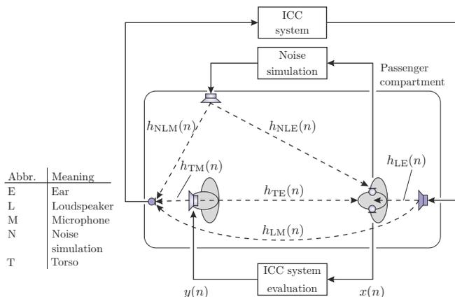
**Figure 1:** Basic structure of an ICC system and the evaluation environment including a necessary noise scenario inside a vehicle [4].
