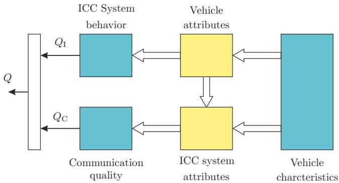
**Figure 3:** Derivation of the overall quality result of the instrumental evaluation according to [9].
