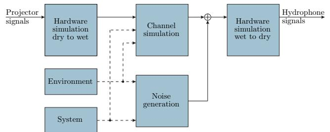
Figure 1: Block diagram of the USE.
