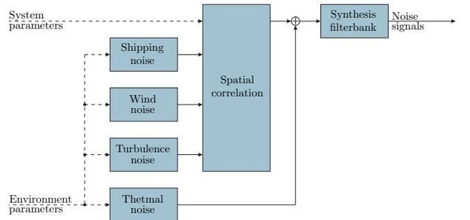
**Figure 7:** Block diagram of the Noise generation module.
