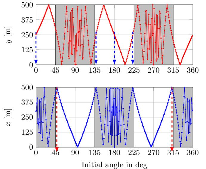
**Figure 5:** Upper: y- and lower: x-values of 361 rays at the x- and y-position of the receiver, respectively, as a function of the initial angle. The transmitter is located at the position (50 m, 250 m) and receiver at the position (500 m, 250 m).
