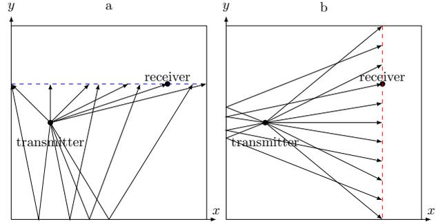
**Figure 4:** Determination of the a: x- and b: y-values for the detection of the eigenrays in the horizontal plane.
