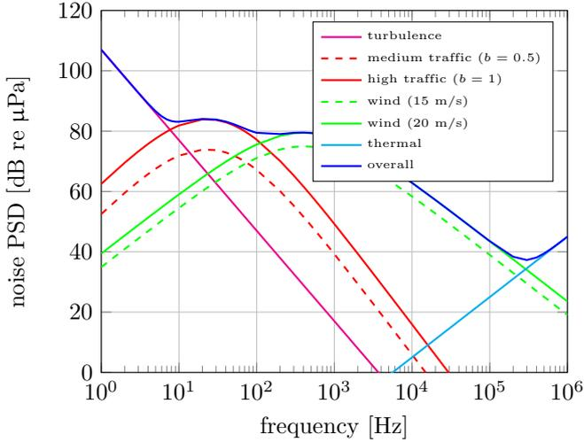
**Figure 8:** Power spectral density of various empirical noise models.
