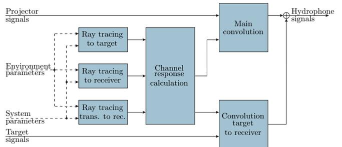
Figure 2: Block diagram of the channel simulation module.
