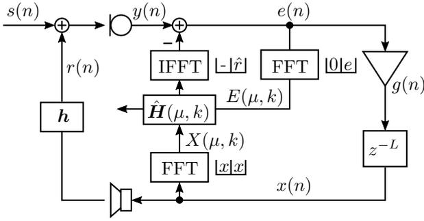
**Figure 2:** Block diagram of the adaptive feedback canceler.
